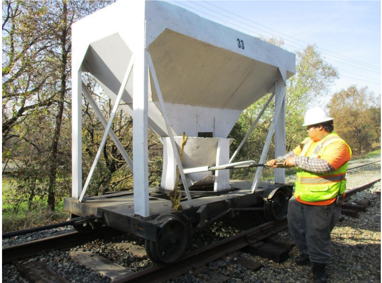
Anthony drops rock from the center-dump ballast hopper
