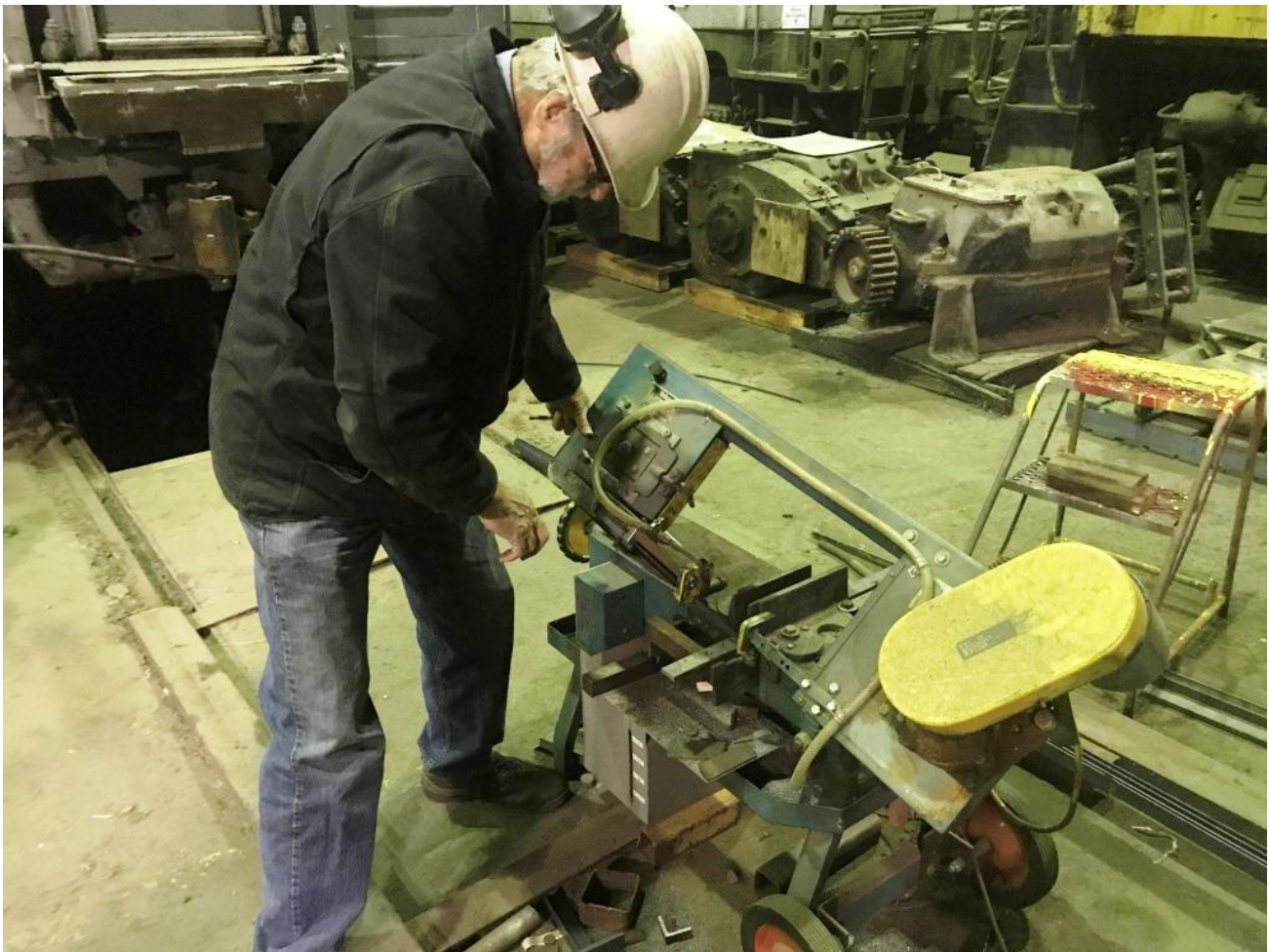
Alan uses the band-saw to cut a shim for the new mounting brackets
