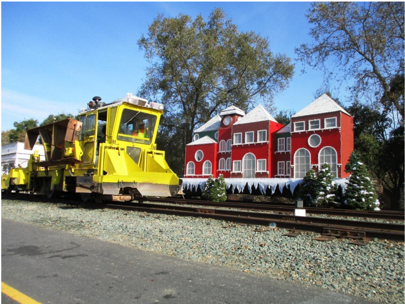
Meanwhile, the ballast regulator passes by an abandoned Santa's Village
