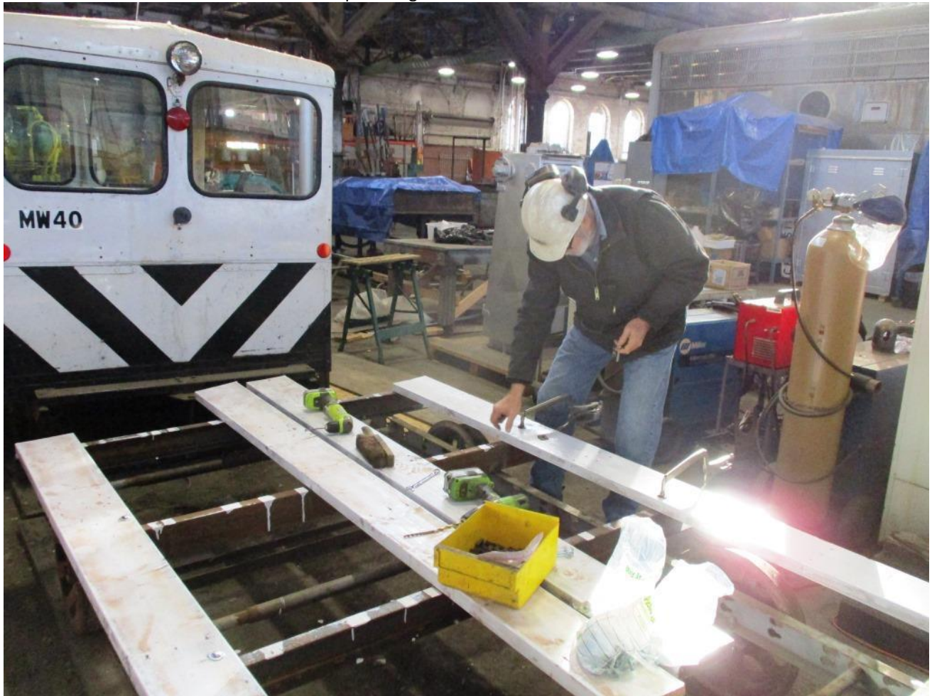
Alan begins the installation of the deck on the hydraulic tool dedicated flatcar
