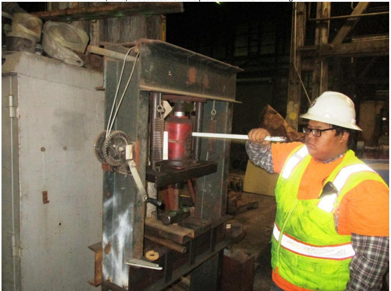
Anthony, using the press, presses out the broken handle from a sledge hammer
